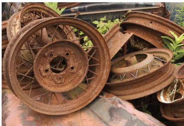
The rusting of these wheel rims is a slow but spontaneous reaction.
