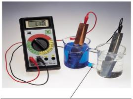
The salt bridge in part (**a**) is replaced by a porous glass disk that allows ions to flow between the anode and cathode compartments but prevents bulk mixing. If  $Cu^{2+}$  crossed the membrane and came into direct contact with zinc, then electrons would be transferred directly and would not flow through the wire.
